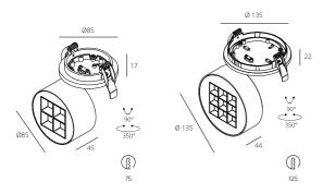
MEGA luminaires create the effect of natural light. Soft white light can act as both the main and an additional source. The rotary mechanism allows you to adjust the direction of light flow, focusing on individual interior items. The body of the product is made in a cylindrical shape with square holes. Inside each of them is a bright LED. Lighting fixtures are suitable for both private and public spaces.
