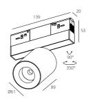
SEJO is a one-of-a-kind spotlight collection that may be mounted on a track. The interior light highlights are created by the ultra-narrow angle of light (only 8°). Instead of a normal reflector, a concentrating (convex) lens is utilized, resulting in a stronger light point. The lighting fixture may be placed anywhere on the track and moved around effortlessly.
