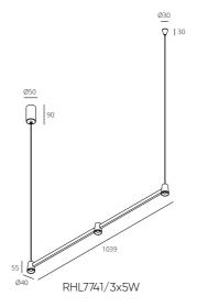
The hanging lighting fixtures of the SANTY series have a modern, minimalist design. The body is made of high-quality aluminum. The lamps are available in two colors. The built-in light source provides visual comfort and prevents glare. Instead of the usual reflector, a lens is used, which allows you to create a powerful directional light flux and provides brighter lighting. In addition, these lamps provide a clear light spot — this makes it easier to emphasize the necessary areas.
