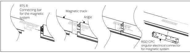
Install the connecting bar in the correct position.
