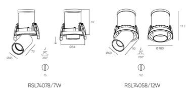
CINI luminaires are available in two capacities: 7W and 12W. A distinctive element of this collection is the spot, which is "hidden" inside the built-in structure. The body of the CINI luminaire is made of durable aluminum, and high-tech, high-brightness LEDs are used as the interior filling, which makes it possible to use the luminaire as the main light source. Thanks to the rotary mechanism, the direction of light flux is easily changed.
