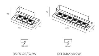
The EVA collection consists of built-in linear luminaires for directional lighting. The frameless design used in this luminaire makes it more elegant and light, and allows you to precisely direct the light flux. Each lens is recessed and separated from neighboring reflectors by a black frame. In addition, this color reduces the number and intensity of flashes. Due to this, the lighting is the most comfortable for perception.
